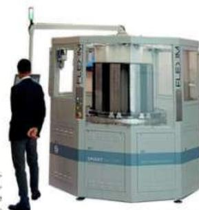
Flexim Open Automation Platform is a scalable production platform allowing the use of a single platform to handle, assemble and process different products. Flexim consists of a machine base, designed to manage more than 80 servos, which is common for all plants and is already designed to accommodate any type of machining station.
